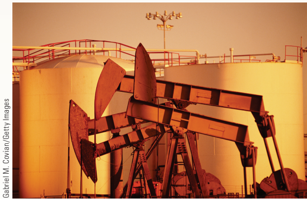
Horizontal beam transfers loads as part of oil well pump
